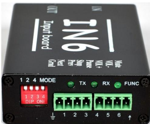
The IN6 input board does not require power supply. The 12 vdc power comes from the RS485 port. If you are using a single IN6 board, use the RJ12 cable to connect the IN side of the RS485 port of the IN6 board into the SR8's RS485 port.
